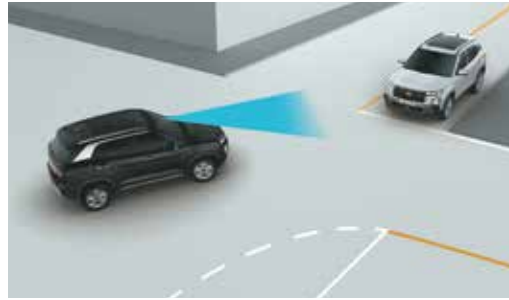
Forward Collision - Avoidance Assist - Junction Turning (FCA-JT)
