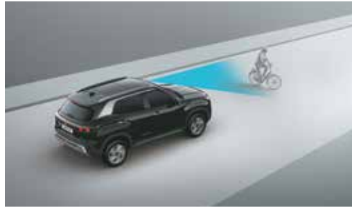
Forward Collision - Avoidance Assist - Cycle (FCA-Cyl)
