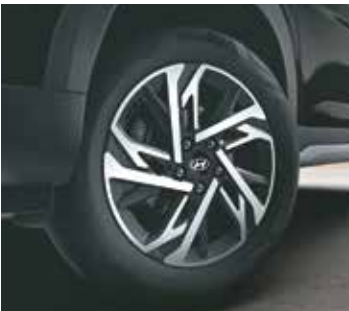
R17 (D=436.6 mm) Diamond cut alloys
